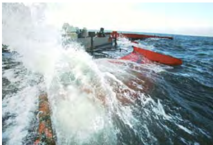
Overtopping device: Wave Dragon
