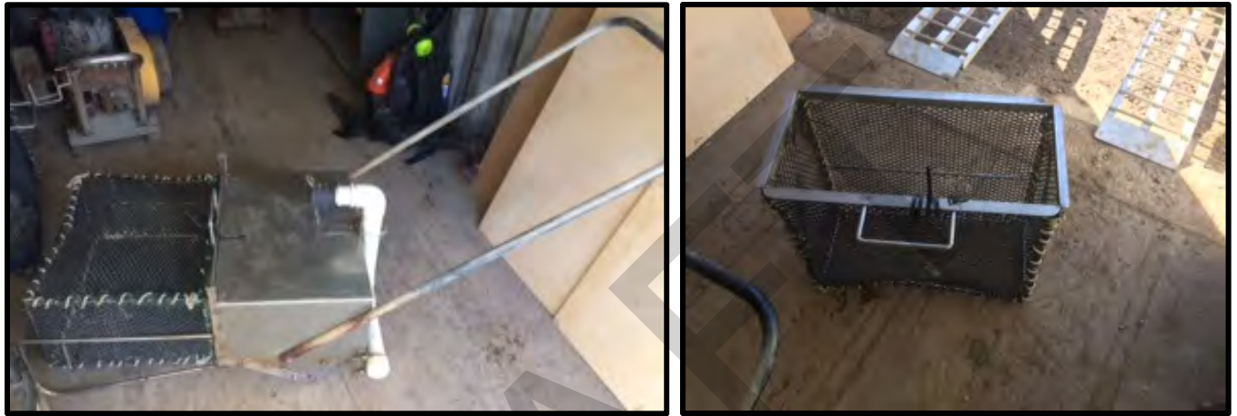
Figure 22. Photograph of Clam Rake and ½-inch Mesh Basket used with the Clam Rake
